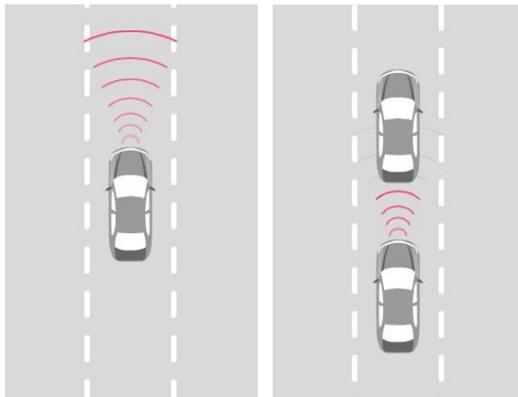
The ACC system, is based on our proprietary 76GHz radar technology. The radar detects objects in its path and monitors both the distance and speed of the vehicle in front. By tracking a preceding vehicle, the ACC system provides automatic acceleration and deceleration to maintain a desired or safe distance. This in turn provides the driver with a safer, more comfortable, and stress free driving experience.
