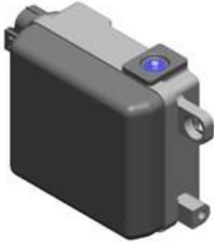
The Elesys Millimeter Wave Radar operates by emitting a 76 GHz radio signal in a predefined direction through a transmitter. The waves reflected by objects located within the radar's detection range are then received back by a receiver module and processed to determine the distance and relative speed of those objects. This information can then be used to maintain safe distance or stop if necessary to avoid collision.
