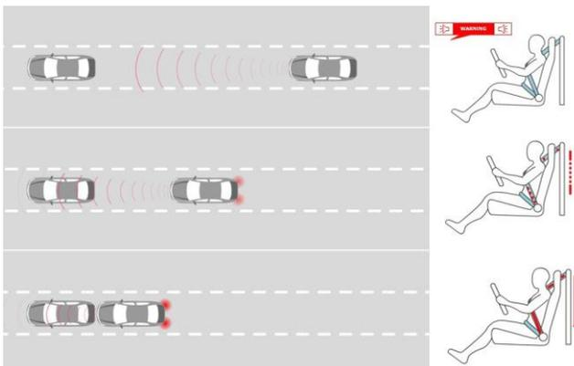
The Elesys Collision Mitigation and Braking System (CMBS) works in conjunction with ACC to provide full braking in emergency situations. CMBS will first alert the driver through an audio and visual warning. Next, it will apply moderate braking to slow the vehicle and engage the E-PreTensioner to “tug” the seat belt to notify the driver. Then, if needed, it will engage stronger braking power to avoid or mitigate the effects of a collision.
